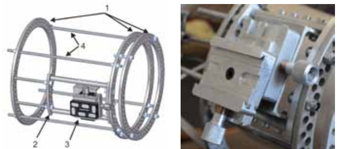
Figure 3. Ilizarov apparatus with fixing system: a) CAD model: 1 – Ilizarov rings, 2 – adaptive guides of fixing system, 3 – coupling unit of fixing system, 4 – Ilizarov ring's rods; b) picture of coupling unit of the fixing system.
