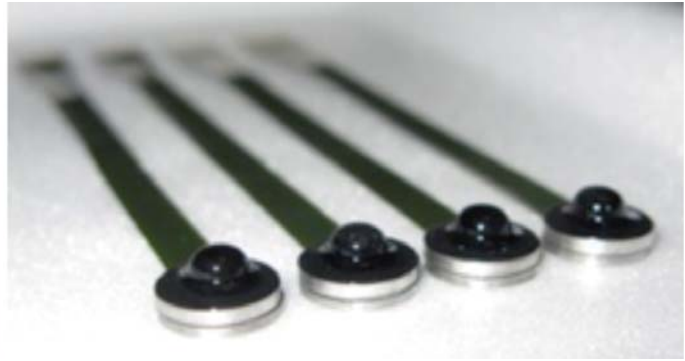
Figure 5. The packaged force sensor for the MIS laparoscopic camera control device mounted on a dedicated flexible PCB and covered by a PDMS cap. The polymer coating is black to eliminate light induced false signals.
