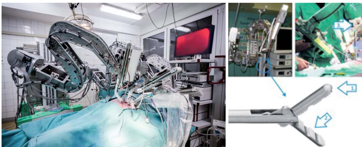
Figure 1. The representation of the proposed applications of the vectorial force sensor in ROBINHEART Minimal Invasive Surgery robot systems
