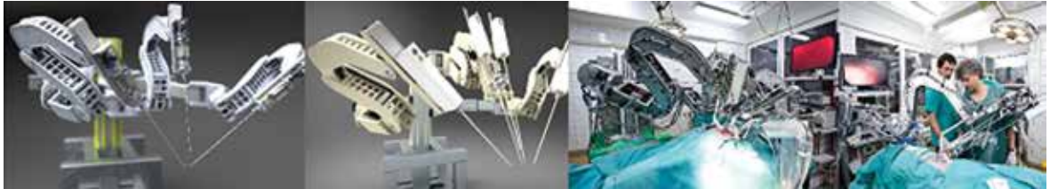
Figure 8. Robin Heart mc^2 – modular robot hardware allows optimal set up into the operation. The robot can work in a set of four tools + endoscope, or as a standalone platform with two tools & endoscope working in the local work area
