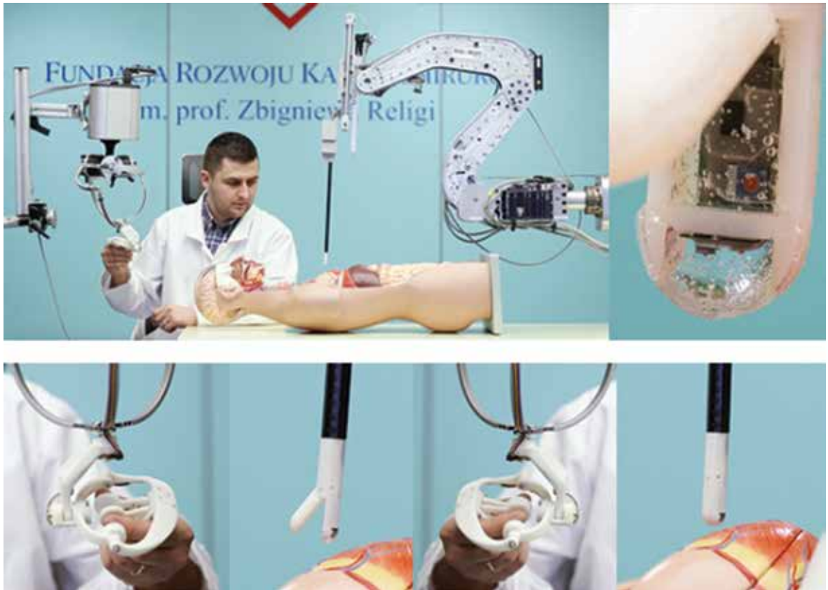
Figure 12. Robot control demonstrator with force feedback. Integration of the Robin Heart robot with the sensory robot tool
