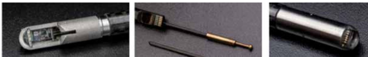
Figure 6. The technology combines composite materials (carbon fiber profiles) with light metal alloys and components made by 3D printing or DLS technology as well as pressure mould elastomer. The ready to use robot integrated laparoscope head with the mechanically manipulated upper jaw is electro-polished (right)
