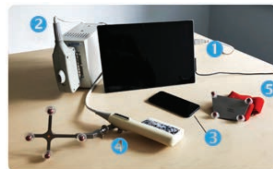
Figure 2. Components of the measuring system (1: Tablet Microsoft Surface Pro 4, 2: Ultrasound device, 3: iPhone 7, 4: Ultrasound probe and adapter with a marker, 5: Marker on a tape)
