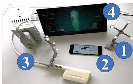
Figure 2. Components of the measurement system: (1) reference rigid body (Aesculap AG, Tuttlingen, Germany), (2) handheld tracking system (iPhone 7, Apple Inc., Cupertino, USA), (3) Ultrasound device (Echo Blaster 128, Telemed, Vilnius, Lithuania) and (4) ultrasound transducer with attached rigid body, (5) central unit (Microsoft Surface Pro 4 tablet)
